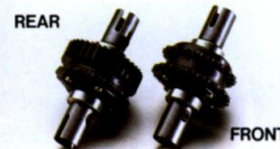
SOUS LA CARROSSERIE TRES STYLEE SE CACHE UNE MECANIQUE DE HAUT NIVEAU! QUATRE ROUES MOTRICES ENTRAINEES PAR CHAINES CARENEES. SUSPENSION TRIANGULEE A LONGUE COURSE. DIFFERENTIELS A ENGRENAGES A L'AVANT ET A L'ARRIERE
