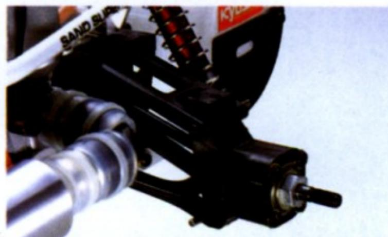
SUSPENSION AVANT A DOUBLE EFFET POUR STABILITE ACCRUE LORS DES SAUTS. BRAS DE SUSPENSION EN NYLON 66EX RENFORCE A LA FIBRE DE VERRE. ROULEMENTS A BILLES SUR TOUTES LES ROUES. DIFFERENTIELS A ENGRENAGES A L'AVANT ET A L'ARRIERE.
